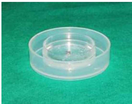
Fig 4. Bracket placed in 35mm petridish containing 5 ml artificial saliva. Then the sample carrier placed in 50mm petridish.
