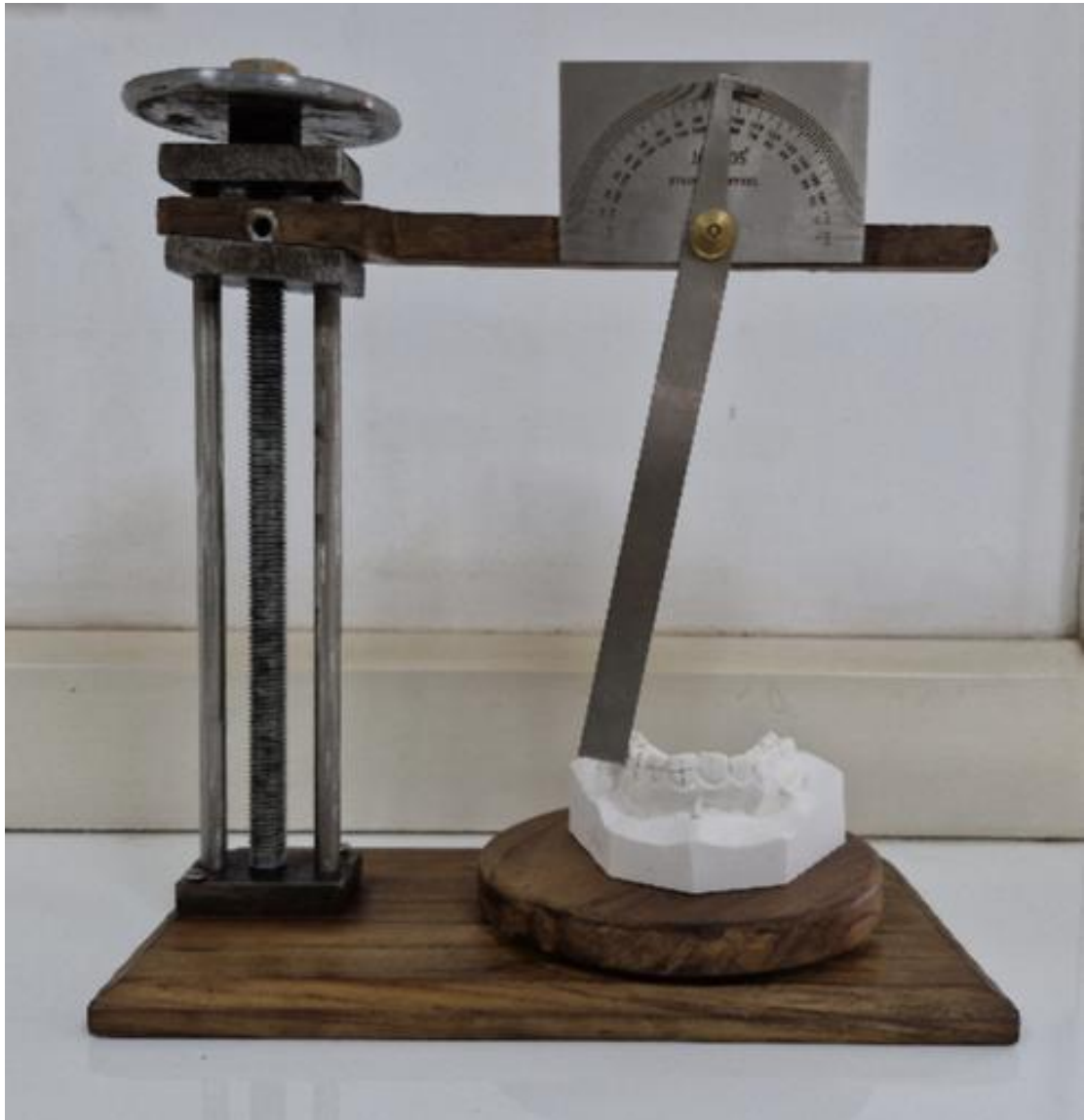
Figure 2: Mounted Angle Protractor measuring crown inclination
