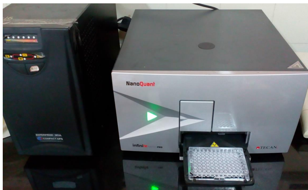
Figure 18: The microplate reader (Tecan Infinite M200) used to measure the optical density.
