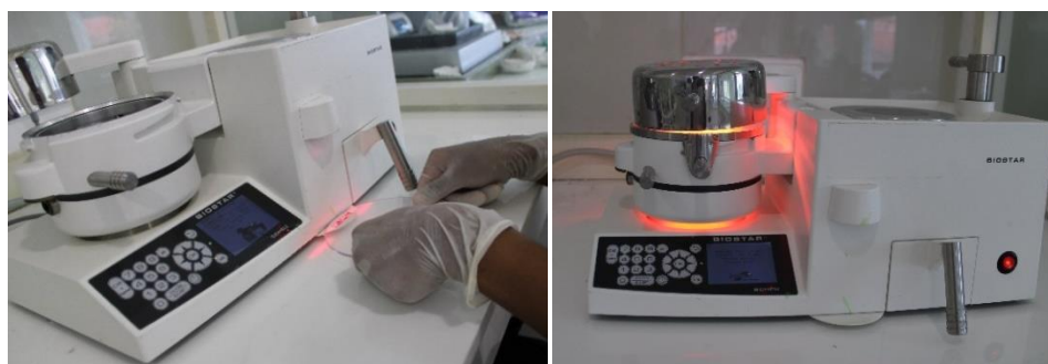
Figure 8, 9: The Biostar (Make:Scheu, Germany, Model: Biostar IV), the equipment which was used in the fabrication of Essix Retainer.
