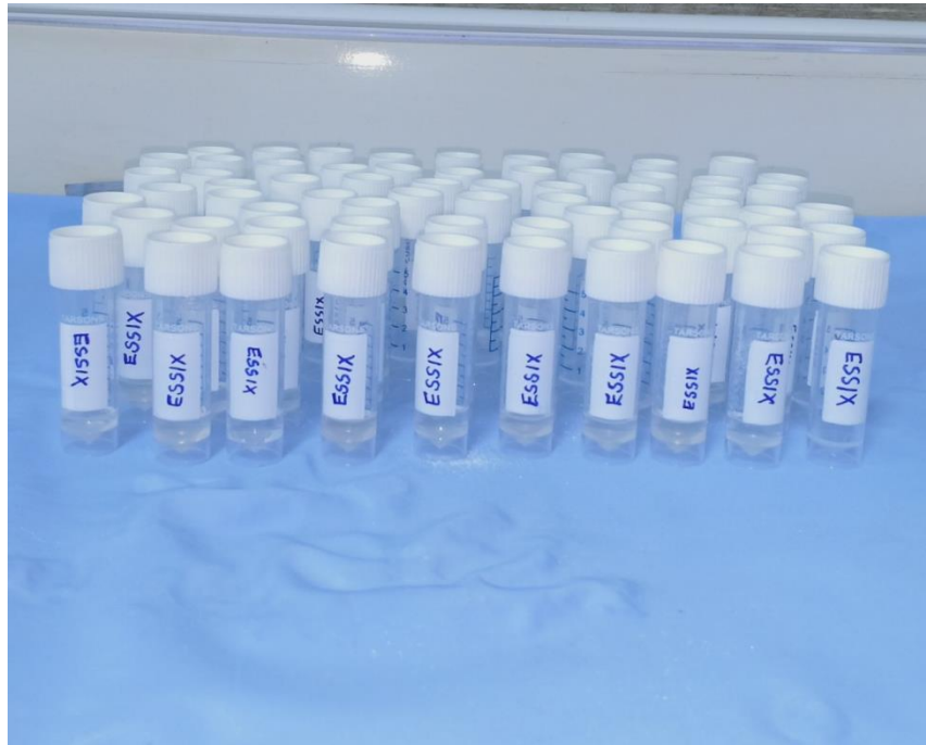
Figure 13: The sterile vials with particulated Essix material soaked in 1 ml artificial saliva.
