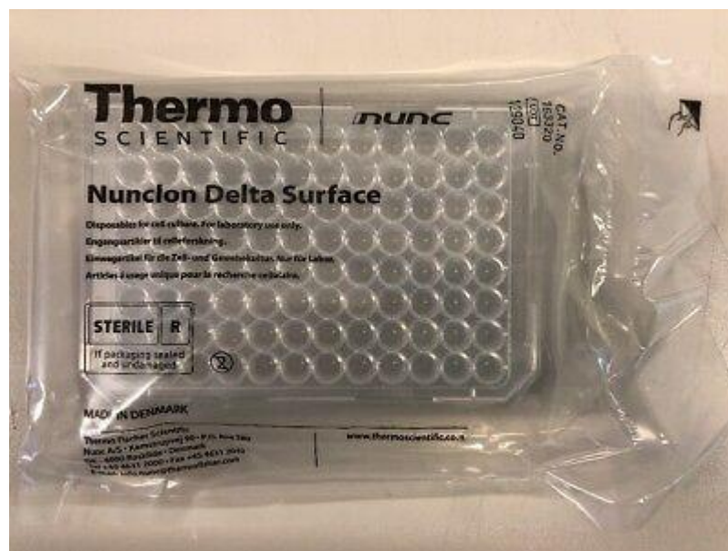
Figure 15: The microplates (Thermo Fisher Scientific-Nunclon 96 Flat Bottom Transparent Polystyrene) used in MTT assay.
