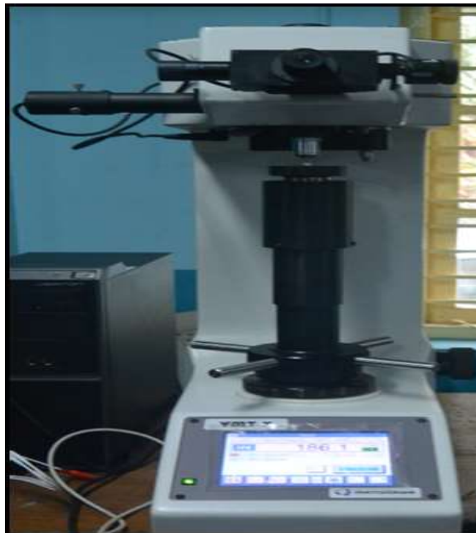
FIG 10: MICRODUROMETER WITH A VICKER'S TYPE DIAMOND PENETRATOR
