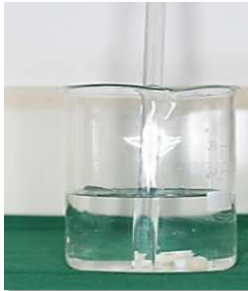
FIG 13: SAMPLES WERE IMMERSED IN 1% CITRIC ACID SOLUTION
