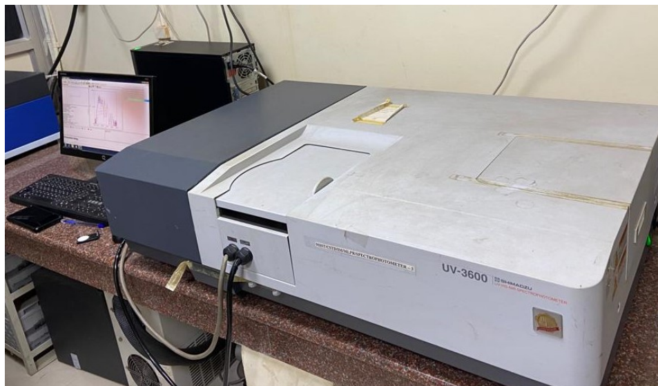
Figure 17: Spectrophotometer for measuring color stability
