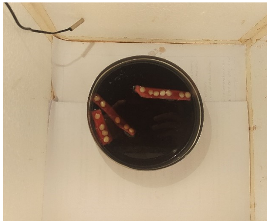
Figure 15: PMMA specimens dipped in coffee in an incubator
