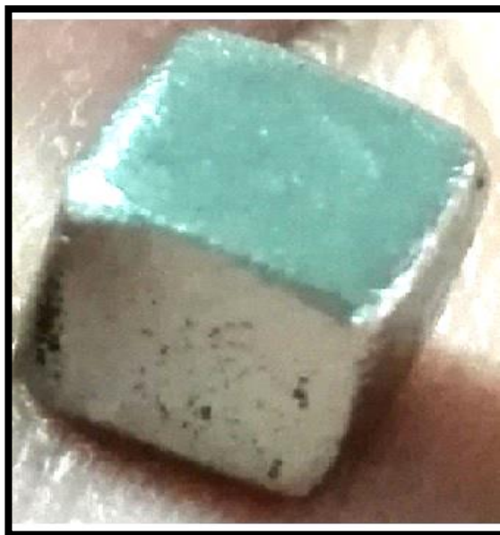
DMLS Co-Cr metal alloy blocks without groove
