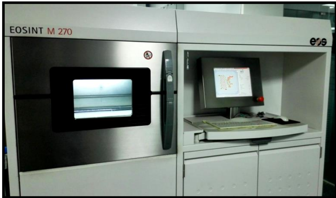
Direct Metal Laser Sintering Unit - EOS EOSINT M 270
