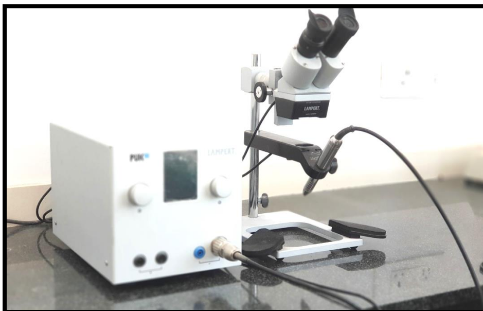
Spot Welding unit - LAMPERT PUK D2
