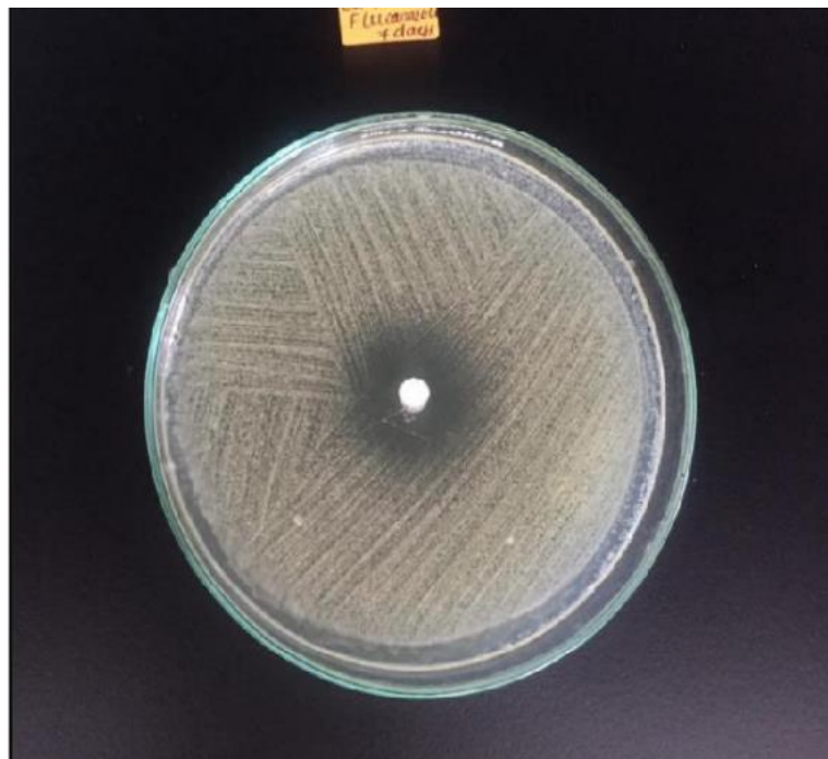
Figure 16: Soft liner disc incorporated with fluconazole showing its activity against Candida albicans standard strain at 7 days
