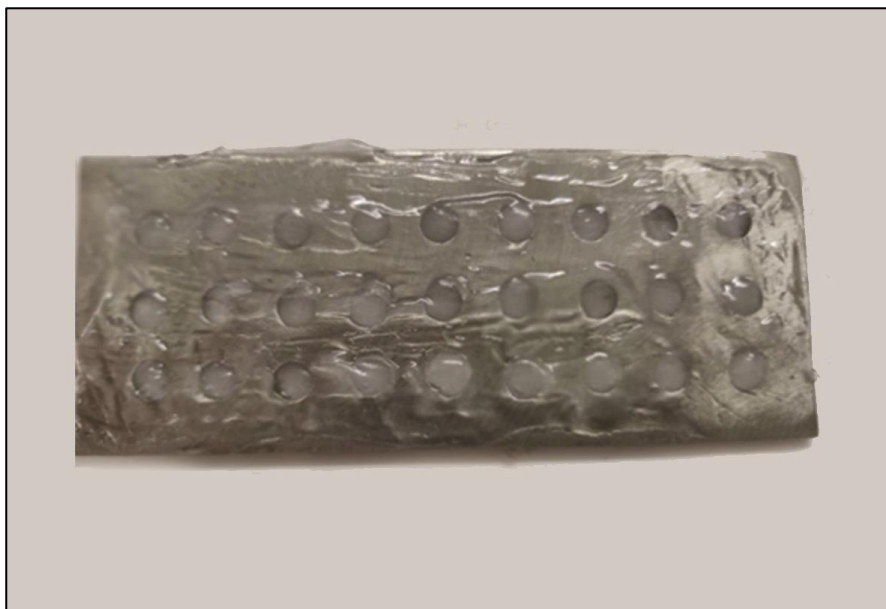
Figure 4 : Pre fabricated stainless steel template filled with the soft liner to which the antifungal agent is added
