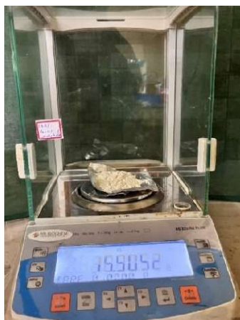
Fig 5 – 15mg of Ferric sulphate weighed on electronic analytic balance
