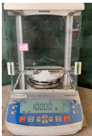
Fig 8 – 100mg of aluminium sulphate weighed on electronic analytic balance
