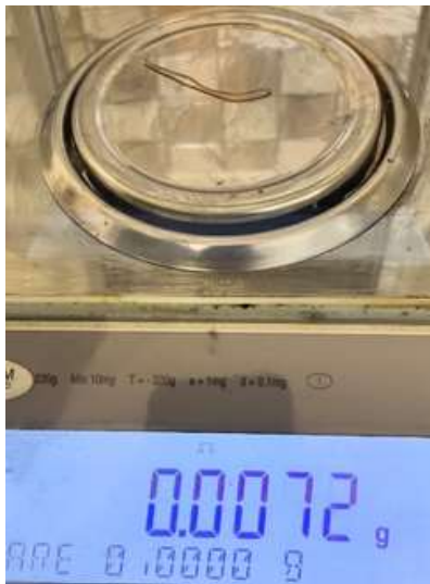
Fig 15 -Dry weight of retraction cord
