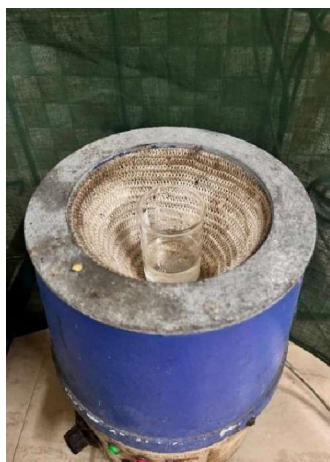
Fig 10 - Aluminium crystals heated around 60°C on heating mantle to accelerate dissolution
