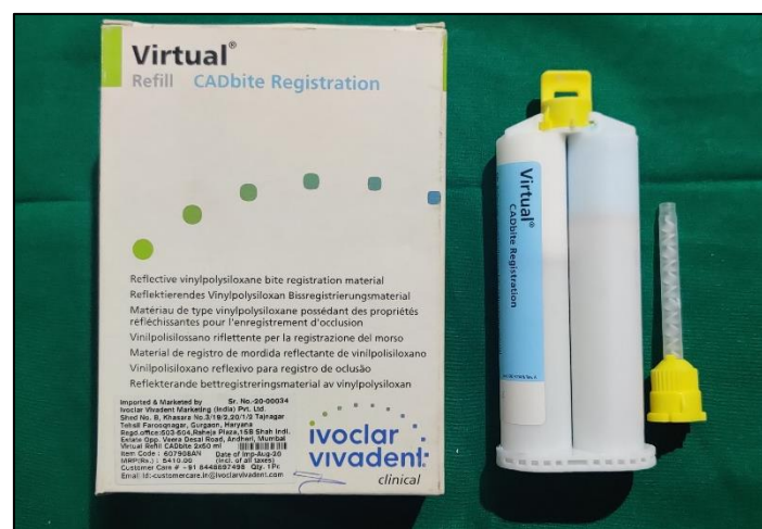
FIG. O4: GROUP A SPECIMEN- IVOCLAR CADBITE POLYVINYL SILOXANE MATERIAL
