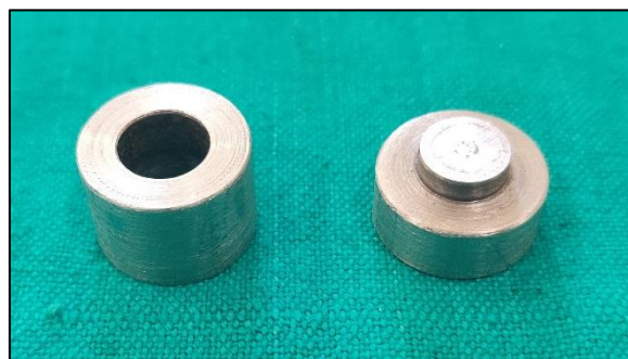
FIG. O3: STAINLESS STEEL DIE FOR EVALUATION COMPRESSION RESISTANCE
