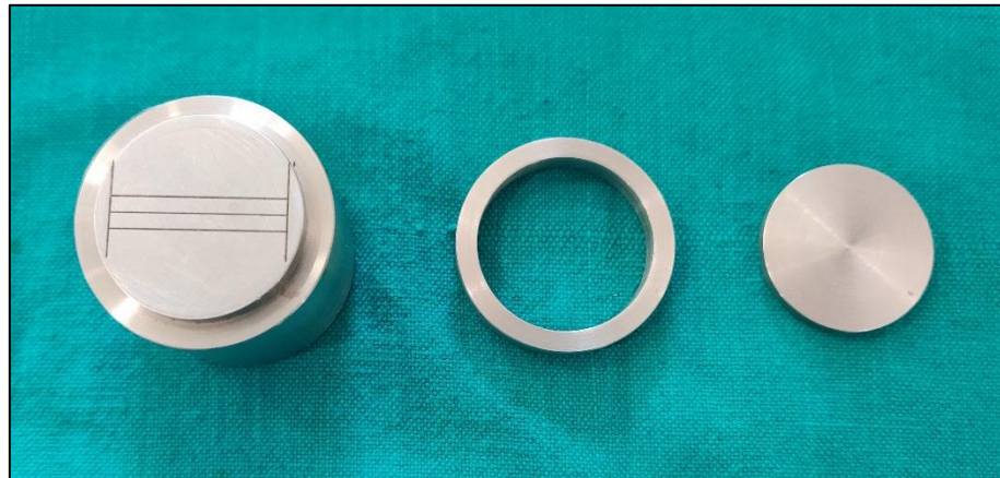
FIG. O2: STAINLESS STEEL DIE FOR EVALUATION OF LINEAR DIMENSIONAL STABILITY (ACCORDING TO ADA SPECIFICATION NO. 19)
