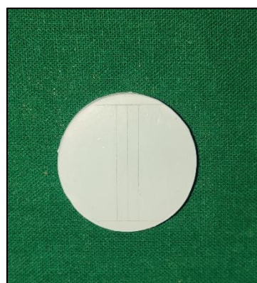
FIG. 12: DEMARKATION OF THE LINES ON SAMPLE PREPARED FOR EVALUATION OF LINEAR DIMENSIONAL STABILITY
