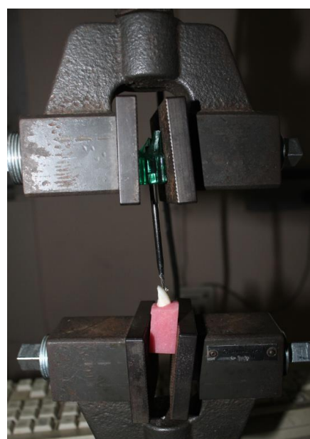
FIG 22: Testing of shear bond strength
