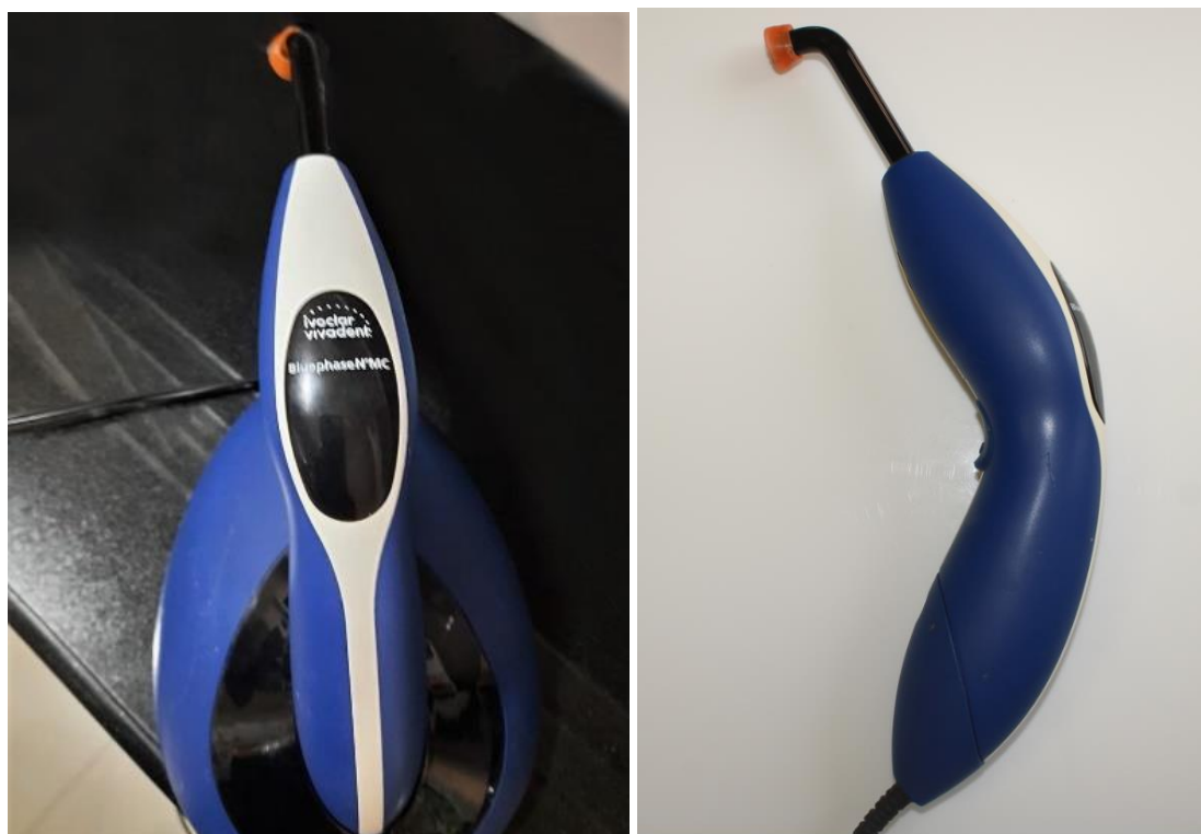
FIG 8: Blue phase LED unit for curing control group samples
